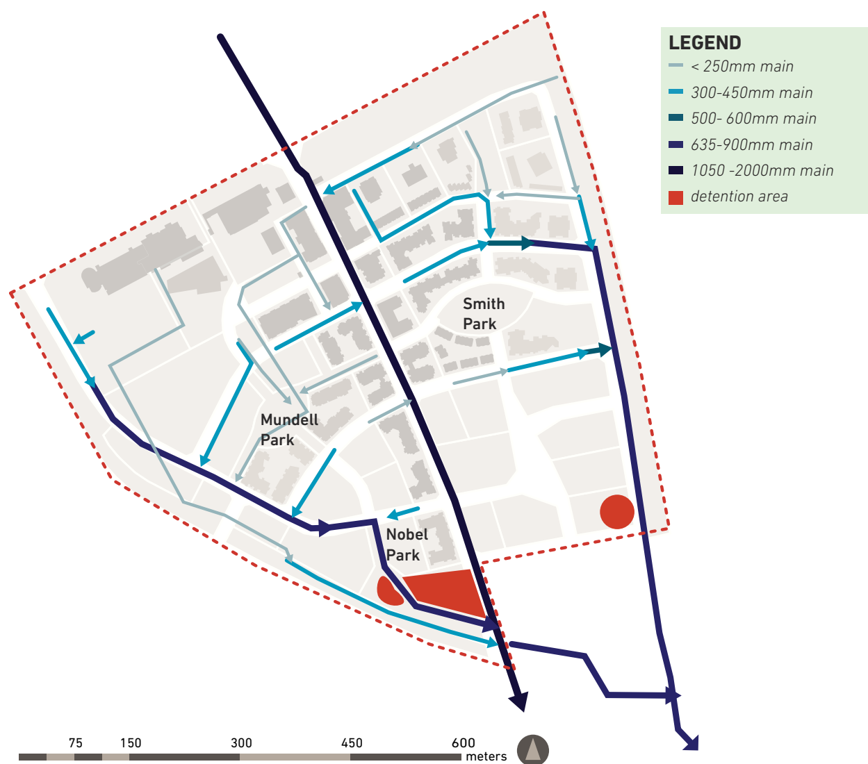
Figure 5.4 Sub-surface drainage system
